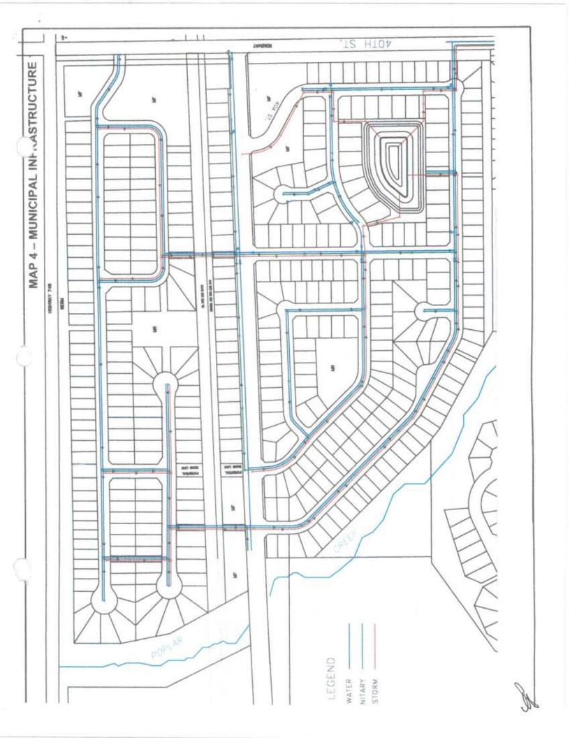
Stormwater management will be provided through storm sewers installed within the road system and public utility lots, flowing into a wet storm pond located in the southeast quadrant of the plan area. This storm pond will allow a controlled realease into the Town's existing storm water system in accordance with requirements of Alberta Environment.
