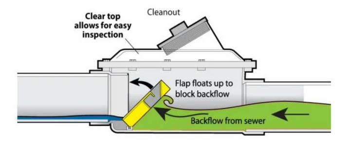
\*The above picture is an example of the typical back-flow preventer used in residential application.
